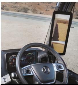
MirrorCam's aerodynamic design can cut fuel consumption by up to 1.3%
