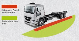
ASGA detects moving objects on the left-hand side of the vehicle, triggering an eye-level warning light to attract the driver's attention to the left-side wing mirrors. If there is a risk of collision, the warning light flashes several times in red. After two seconds, it remains permanently illuminated in red and, in the event of an imminent collision, a warning tone also sounds.
