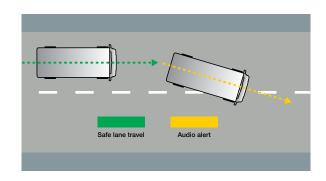
**LDWS** operates at speeds over 60km/h to reduce the risk of lane departure accidents caused by distraction or fatigue.
