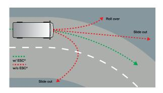
**ESC** employs a steering sensor and yaw rate sensor to detect loss of control.
