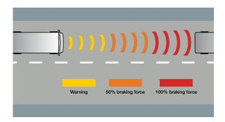
**AEBS** helps to avoid or mitigate collisions with pedestrians and other vehicles by using a radar to monitor the road ahead.
