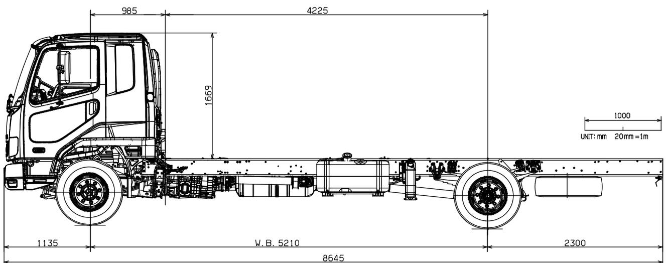
Scale = 1:50 (20mm = 1 metre). This scale is accurate when used on the original spec sheet, be aware that enlarging these illustrations can alter the scale and cause incorrect measurements. Fuso New Zealand and its authorised dealers always recommend customers seek professional advice from independent sources before commencing any engineering activities.
