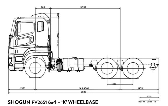
Scale = 1:50 (20mm = 1 metre). This scale is accurate when used on the original spec sheet, be aware that enlarging these illustrations can alter the scale and cause incorrect measurements. Fuso New Zealand and its authorised dealers always recommend customers seek professional advice from independent
