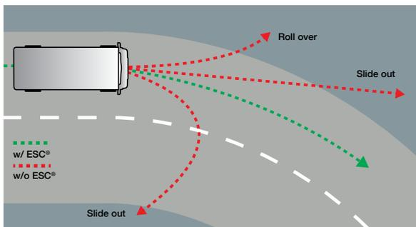
**ESC** employs a steering sensor and yaw rate sensor to detect loss of control.
