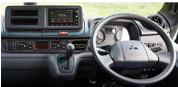
An on-dash screen relays images from the rear-mounted reversing camera and works with Apple CarPlay or Android Auto for hands-free talking text-to-speech functionality.
